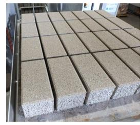
(c) Carbonation-cured low-carbon IL blocks
