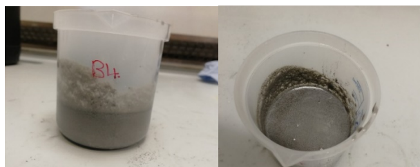
Figure 3 – Sample B4, 40 wt% of Nevastane potassium geopolymer with a ‘shiny’ layer on the surface of the cement.
