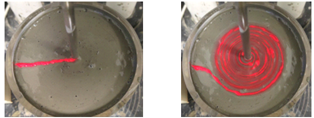
Fig. 2 Distinguish of shear zone and plug zone by pigment (Series No.2, 15 r/min)
