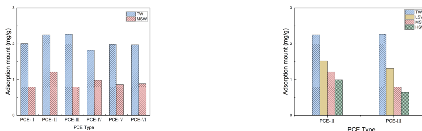
(a) Effect of different PCEs in TW and MSW (b) Effect of different salinity Fig. 3. Effect of PCE type and SW salinity on adsorption amount of the cement paste
