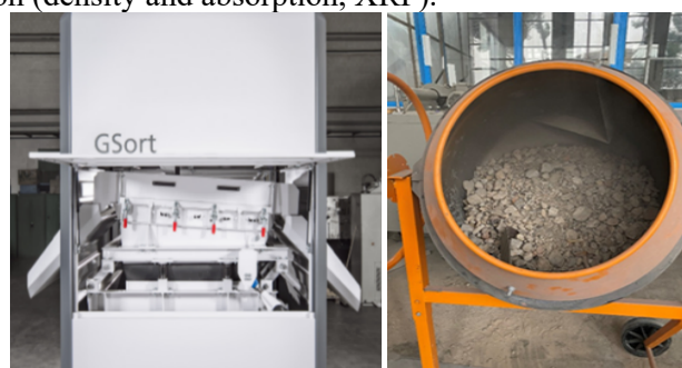
Figure 1. (Left) Densimetric table – ALLGAIERMogensen; (Right) Abrasion in concrete mixer - IETcc.
