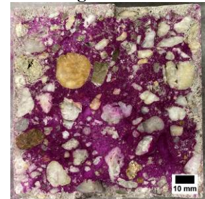
Figure 3: Carbonation after 800 d storage in 1 vol.% \text{CO}_2
