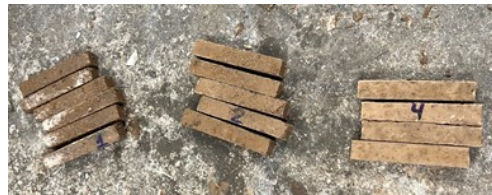
Fig. 1 Physical aspect of MKPCs pastes prepared with different M/P ratios (efflorescences are detected at M/P=1)
