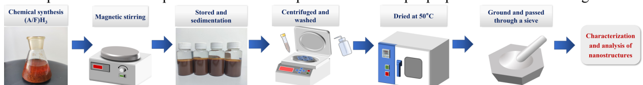
Fig. 1 Procedure for the preparation of Al-substituted ferric hydroxide
