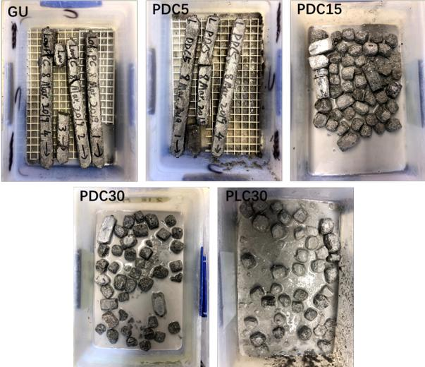
Fig. 2 Visual condition of mortar bars immersed in 5% Na<sub>2</sub>SO<sub>4</sub> solution at 5°C for 150 days
