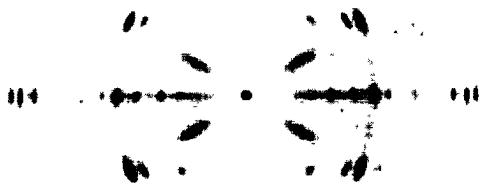
Figure 2: Rotation photograph of crystal of \gamma -C 2 S obtained by heating an afwillite crystal at 650°C.
