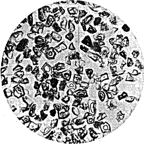
Figure 9: Granulated slag "k" (8 per cent \text{Al}_2\text{O}_3 ). Having been shaken 55\frac{1}{2} hours in 10 per cent ammonium citrate. Ordinary light. Magnification \times 67 .
