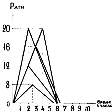
FIGURE 13. "Peak-regime" influence on hardening of cement mortar of the composition 1:3 of plastic consistency.
