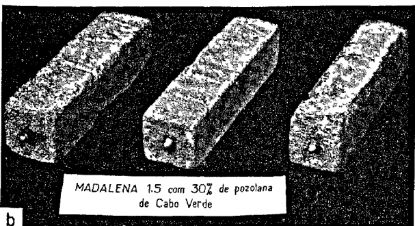
FIGURE 2. Portland cement and pozzolan mortar prisms of granitic aggregate maintained in sea water.
