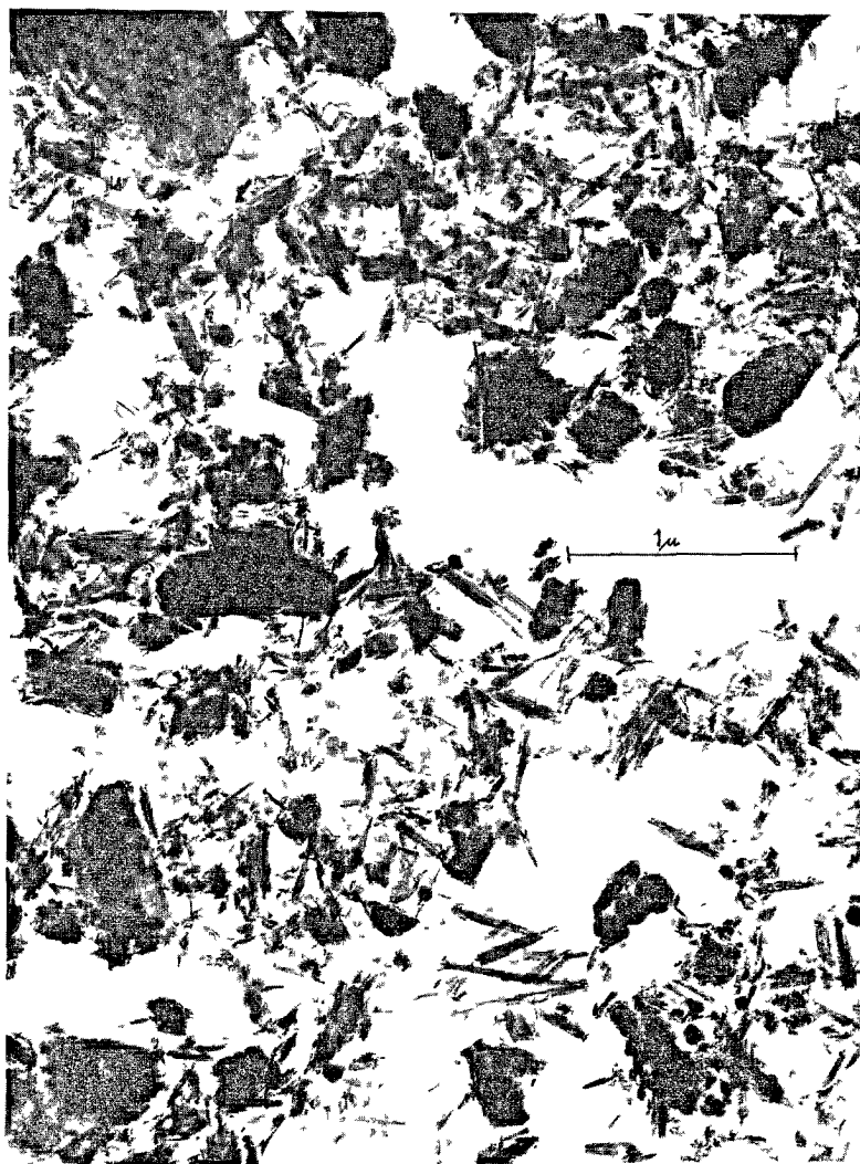
FIGURE 4. Electron micrograph of hydrated C_3S , w/c=0.5 ; duration of hydration, 1 month; hydration temperature, 30^\circ C ; average length of calcium silicate hydrate crystals, 5,000\text{\AA} .
