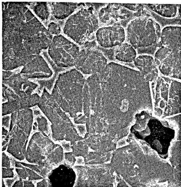
Fig. 43. Scanning electron microscopic photograph of etched surface of N_2 clinker.
