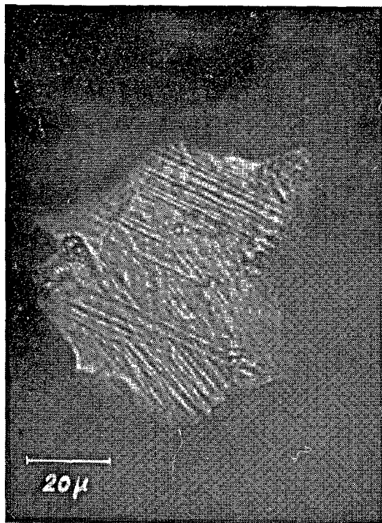
Fig. 30. Transmitted light microscopic photograph of belite grain containing \alpha C_2S
