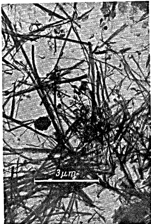
Fig. 8. Electron micrograph of a C_3S - C_3G -paste hardened 1 day w/c = 0.50 (carbon replica) C_3G = tricalcium germanate = 3CaO \cdot GeO_2
