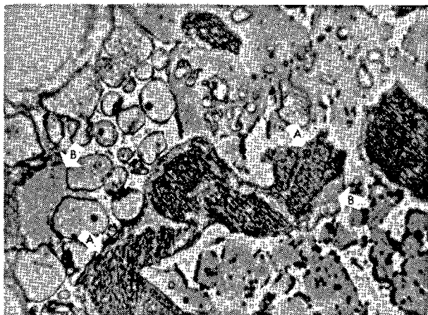
Photo 1. This shows alkali sulphate, arrowed A, infilling irregular pores in the clinker and is thus clearly one of the last phases to crystallise. It occurs here as small oriented crystals, etched a dark colour with hydrofluoric acid vapour. Interpenetration of the embedding plastic resin, arrowed B, used during specimen preparation, indicates volume changes during cooling. Characteristically the alkali sulphate is surrounded by a halo of unetched clinker.
