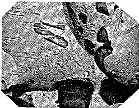
Fig. 6. Etching figures of crystals C 3 S-Magn. × 15000
