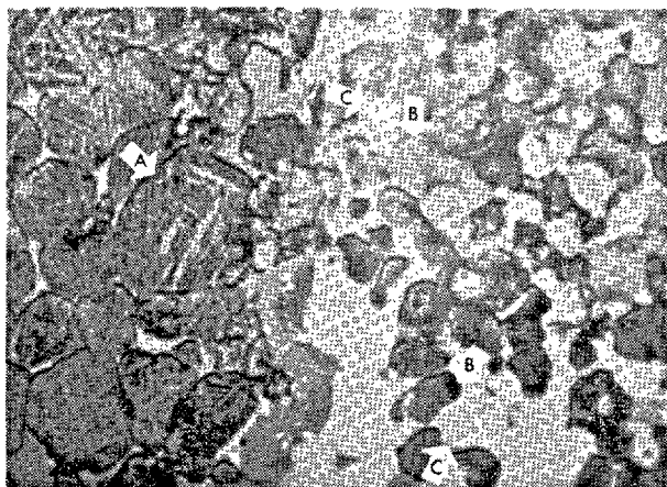
Photo 5. Both the normal belite, arrowed A, and the alkali stabilised belite, arrowed B, are illustrated here. The coexistence of alkali modified belite in contact with free lime crystals, arrowed C, indicates the considerable stability of the alkaline belite inhibiting its assimilation of further lime to form alite.
