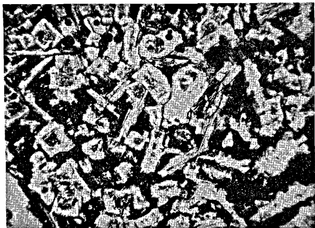
Photo 2. Porphyritic texture of slow cooling slag.
