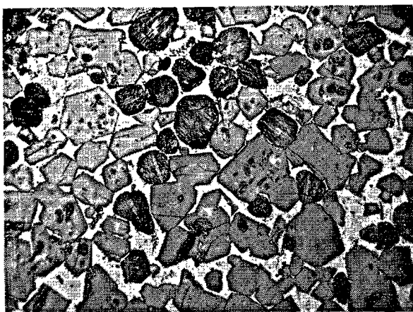
Fig. 1. Photomicrograph of portland cement clinker: the alite crystals are pseudo-hexagonal, the belite grains rounded and striated. The interstitial phase lies between the C_3S and C_2S crystals. Terrier and Hormain (105).
