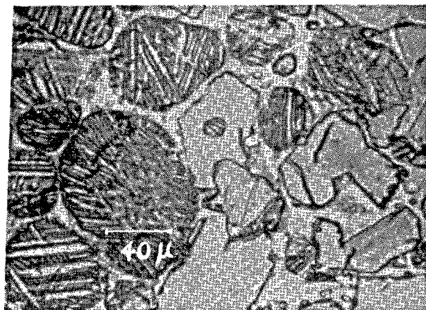
Fig. 33. Reflected light microscopic photograph of alite and type I belite etched with \text{HNO}_3 -alcohol.
