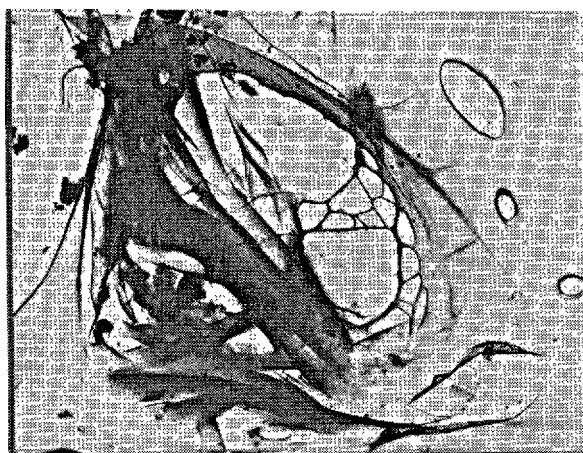
Fig. 14. Electron micrograph of \text{C}_3\text{S} (w/c = 0.44) after seven days
