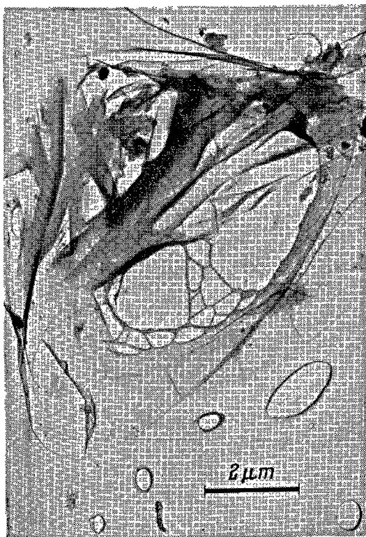
Fig. 11. Electron micrograph of a C_3S -paste hardened 7 days with addition of a retarder w/c = 0.44 (carbon replica)
