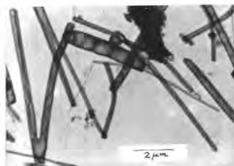
Figure 6 TEM micrographs of synthetic C_3A (+20% gypsum) hydrated for 15 minutes at w/c 0.6 showing the presence of both hollow and solid Aft fibres.
