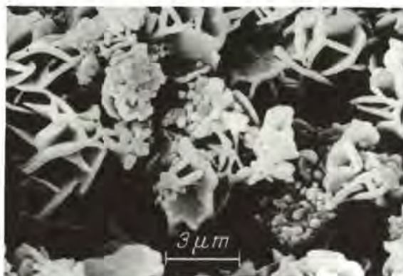
Figure 3: Structure of paste from ground Portland cement clinker without addition of gypsum 30 minutes after mixing
