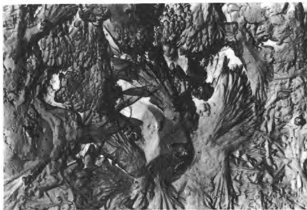
Fig.5. (CaO). 24 h of Hydration. Electron Microscope X14000
