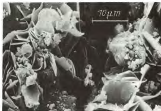
Figure 6: Structure of Portland cement paste with a sulfate supply which is too low
