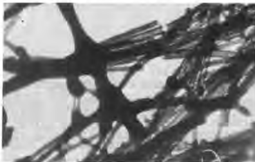
Fig.3. Skeleton from interwoven and intergrown pulled crystals of ettringite (X4000)
