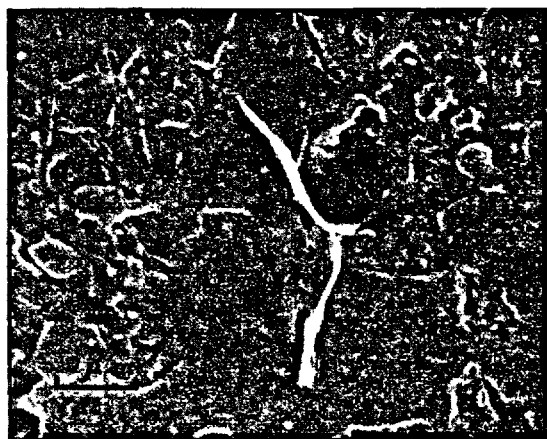
Fig. 6.- Devitrified C_{12}A_7 glass annealed at 1300^{\circ}\text{C} for two hours and subsequently hydrated during half a minute. SEM.
