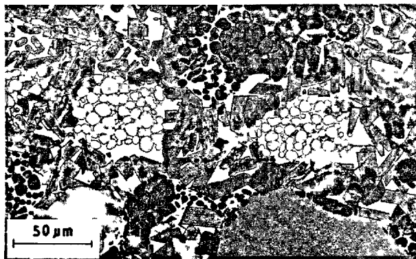
Fig. 3 - Free \text{CaC} agglomerations in C 2 clinker, firing at 1400 °C, 1 minute. Phases according to blackening of photograph: Interstitial mass, free \text{CaO} , alite, belite. Large homogenous area - epoxide. ( \text{CH}_3\text{COOH} vapour)
