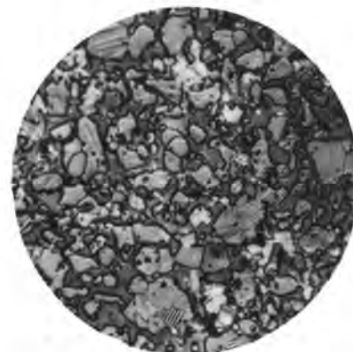
FIG. 3: \text{C}_{2.72}\text{N}_{0.28}\text{A} quenched from 400^{\circ}\text{C} - Nital - 450X
