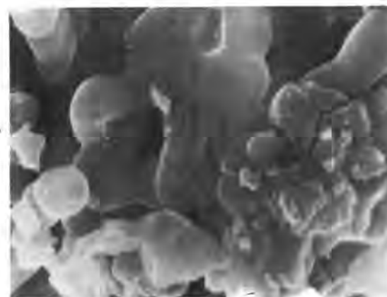
Fig.2. The surface of the mineral NC_8A_3 before hydration (x 20 000).
