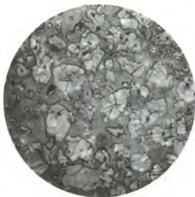
FIG. 6: C_{2.76}N_{0.24}A cooled at room temperature - Nital 450X
