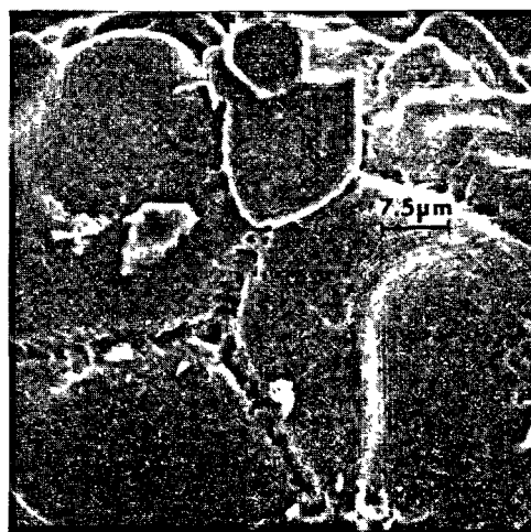
Fig. 7 - Coarseness and secondary crystallization of the belite grains of the second clinker
