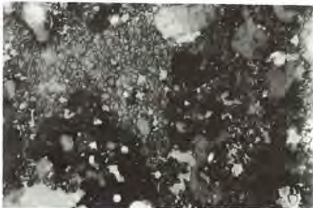
Fig.1 - Reflected light microscopic photograph of normal clinker burnt with CaCl_2 admixture, etched with 1-per cent solution of HNO_3 - alcohol. Shows alite crystals and clusters of belite crystals. Enlarged 800 x.
