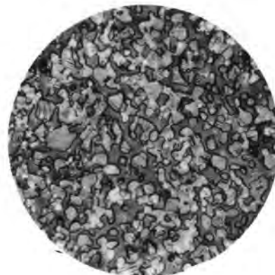
FIG. 12: C_{2.66}N_{0.33}A quenched from 400°C - Nital - 450X
