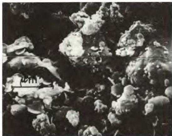
Fig. 4 - Fracture surface of hardened paste No. 1.
