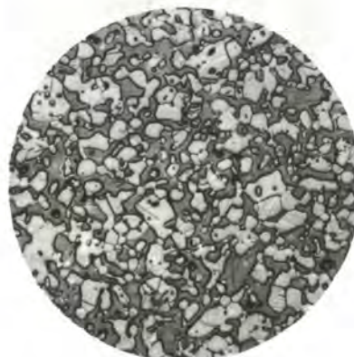
FIG. 9: C_{2.74}N_{0.26}A quenched from 475°C - Nital - 450X
