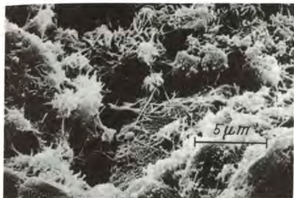
Figure 5: Structure of paste from ground Portland cement clinker with addition of gypsum 4 hours after mixing
