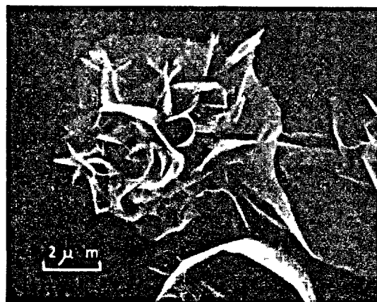
Fig. 7.- Devitrified C_{12}A_7 glass annealed at 1300^{\circ}\text{C} for two hours and subsequently hydrated during half a minute. SEM.
