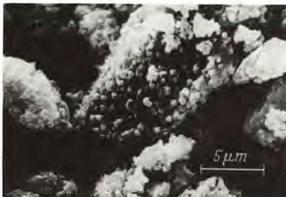
Figure 4: Structure of paste from ground Portland cement clinker with addition of gypsum 30 minutes after mixing
