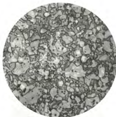
FIG. 8: C_{2.74}N_{0.26}A quenched from 450°C - Nital - 450X
