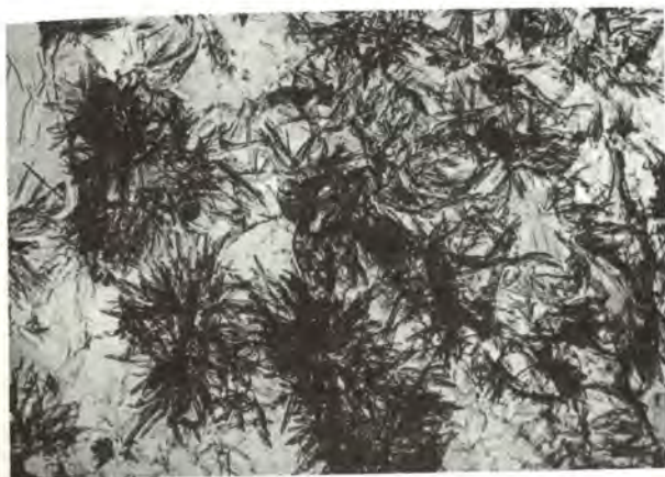
Fig.2. (CaO). 6h of Hydration. Electron Microscope, X10000
