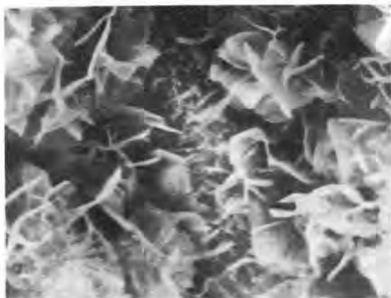
Fig.4. The surface of C_3A after 5 seconds of hydration in the system C_3A-CaSO_4 \cdot 2H_2O-H_2O (x 20 000).
