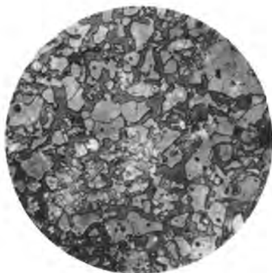
FIG. 1: \text{C}_{2.78}\text{N}_{0.22}\text{A} quenched from 400^{\circ}\text{C} - Nital - 450X
