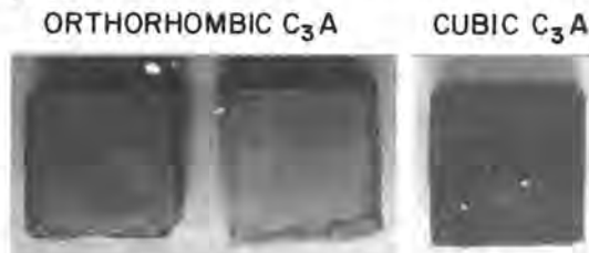
FIG. 3 CEMENT PASTE CUBES AFTER 28 DAYS SULFATE IMMERSION
