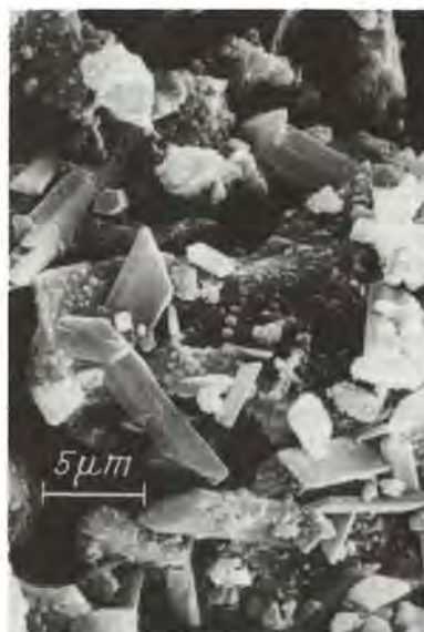
Figure 7: Structure of Portland cement paste with a sulfate supply which is too high
