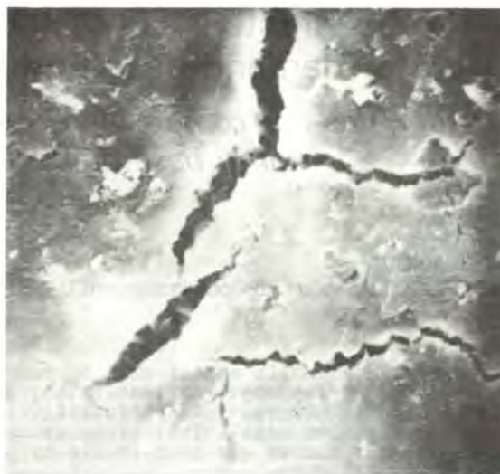
Fig. 4. The microcracks pattern on the bottom of capillary pore in phase V. x 2500. The cracks plane is parallel to the trajectory of fracture
