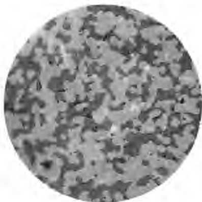
FIG. 15: C 2.66 N 0.33 A quenched from 1350°C - not etched 450X
