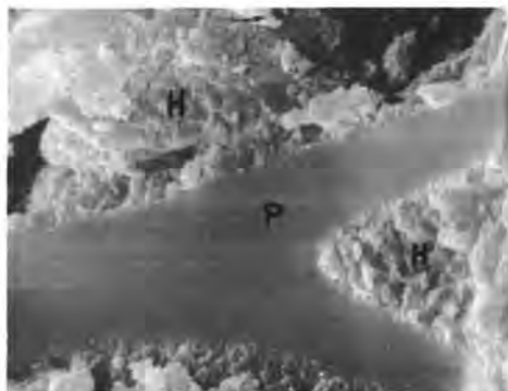
Fig. 9.: Ph_1 M x 10000, Ph_2 M x 10000 Ph_3 M x 10000 Ph_4 M x 10000 Hydrated cement paste ( P_1 +40% S.e) cured in water at 18 \pm 2^\circ C for 1 year.
