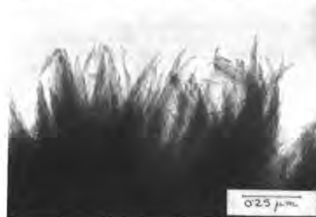
Figure 4. TEM micrograph of synthetic C_3S hydrated for 1 day at w/c 0.6 illustrating the crumpled foil-fibrillar C-S-H morphology.
